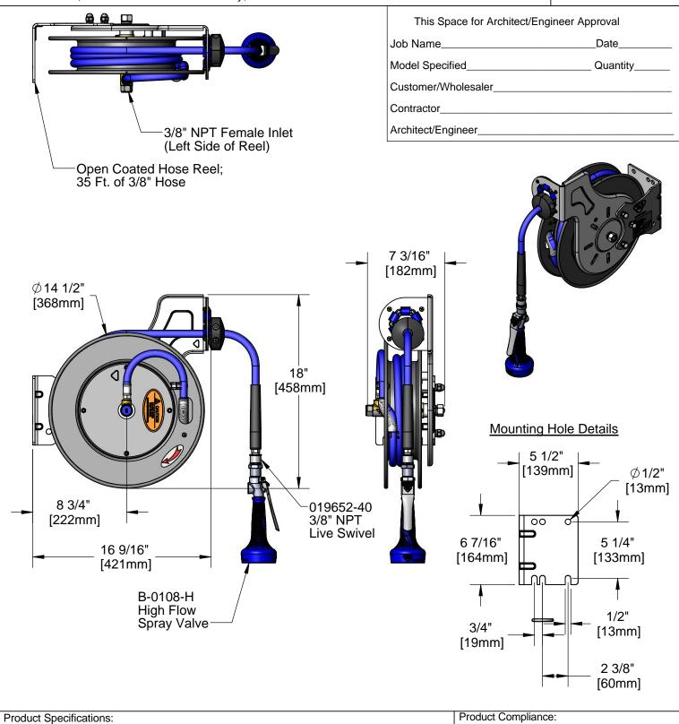
3/8" x 35 Ft. Open Coated Reel w/ High Flow Spray Valve & Swivel
